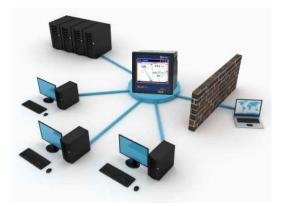
Applications in which data recorded by one device are handled by more than one person, or where the data are important in several process points, can be also implemented based on data downloading using the DAQ Manager. Several computers with an installed software can successfully download data from the same MultiCon recorder at the same time.
