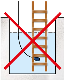
Image 4. Take care to ensure the free movement of the float.
