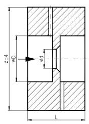
according to the relevant standards (ISO 5167, ASME MFC-3M etc.). The plate type is chosen based on the specific process conditions. The orifice plate edge is usually manufactured from a wear-resistant material like stainless steel. The material of the carrier ring can be equivalent to the pipe material.
