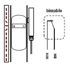
As standard, the magnetic switch is mounted on the outside of the stand pipe opposite the indication rail. See adjacent drawing.
