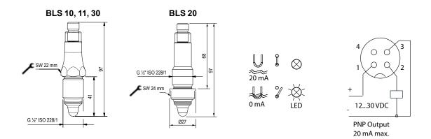
The tip of the sensor is made of PEEK plastic. The sensor works on the principle of frequencysweep technology. The sensor output can be switched from digital to pulse width modulation (PWM). The sensor recognizes different media and can therefore be used for media separation. The analysis of the PWM signal must be done in the connected control unit (PLC).
